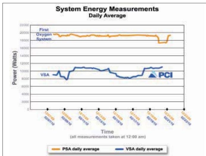
\*Fluke Power Meter data recorded for both the PSA and VSA systems
